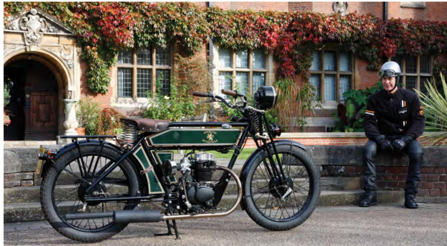
Honda's engineers would doubtless be fascinated to see the CG engine they designed bolted into the Sterling's steel frame, whose top tube runs across the top of the flat-sided, nine-litre aluminium fuel tank. The aircooled, pushrod-operated engine breathes in through a Keihin-replica Keima carburettor, out through a fully catalysed stainless steel exhaust, and produces a claimed maximum of 14bhp at 6000rpm.
