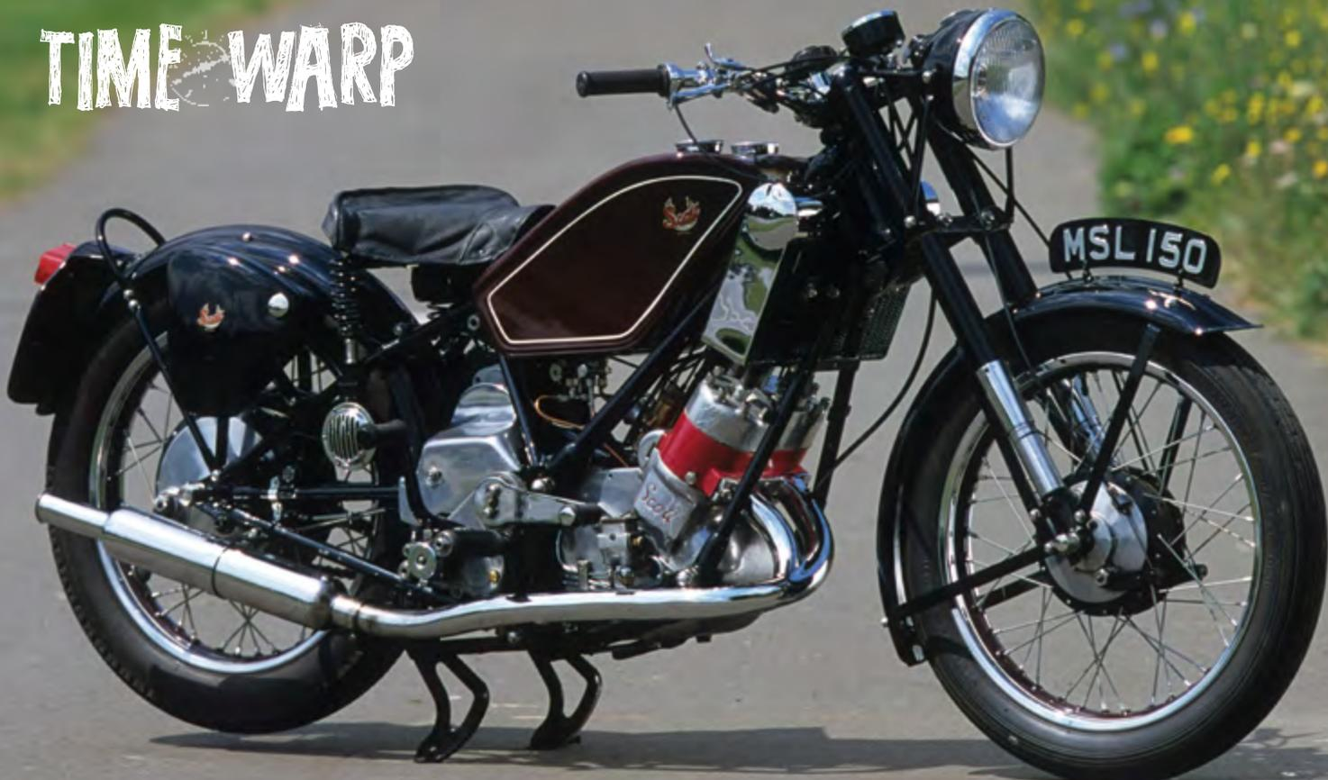
Handling was stable and steady, needing little help from the friction damper. At about 185kg the Flying Squirrel was not particularly light, and its blend of 19-inch wheels and period geometry meant it steered slowly. The wide bars gave plenty of leverage, though they tangled with my knees on full lock during slow-speed maneuvers.
